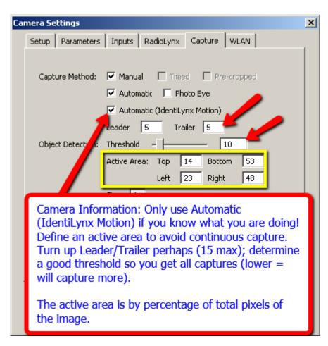
A lower number under threshold makes the camera more sensitive. It is the percentage of change in image it must see before it says "hey I'm supposed to be taking a picture". A higher number makes it less sensitive. So for example if you are on a course with blowing leaves, snow or rain, you might want to try a higher number. If you have a still area, a higher number might be okay.
